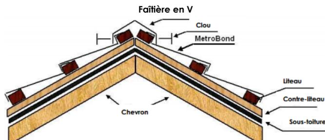
**Fig. 27–** tuiles METROTILE® BOND, METROTILE® BOND 7-PA, METROTILE® ROMAN, METROTILE® CLASSIC, METROTILE® SHAKE, METROTILE® WOODSHAKE, METROTILE® MISTRAL, METROTILE® MISTRAL, METROTILE® ROMANA, METROTILE® GALLO et METROTILE® ELEGANTA – faîtière demi-ronde
