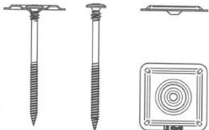
Fig. 1- Vis LR ETANCO EVDF 2C + plaque LR ETANCO 40X40
