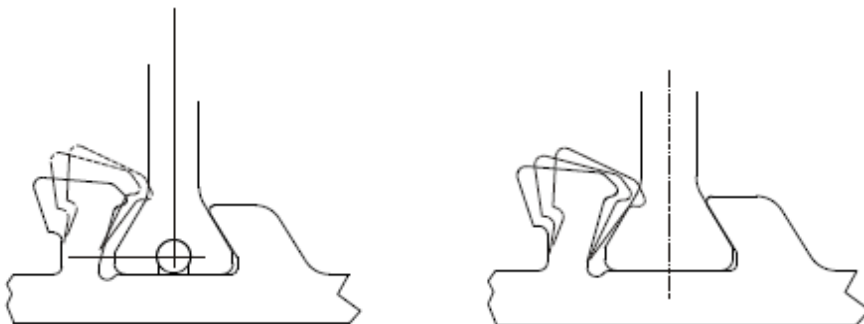
Fig. 2 Example of strip installation
