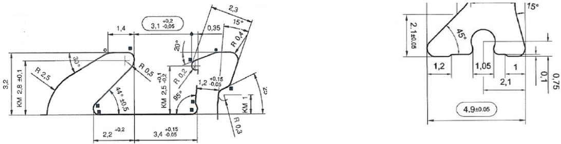
Figur 2 – Coupures thermiques
