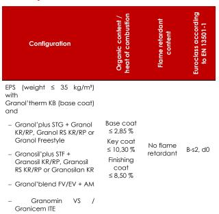
Note: A European reference fire scenario has not been laid down for facades. In some Member States, the classification of ETICS according to EN 13501-1 might not be sufficient for the use in facades. An additional assessment of ETICS according to national provisions (e.g. on the basis of a large-scale test) might be necessary to comply with Member State regulations, until the existing European classification system has been completed.
