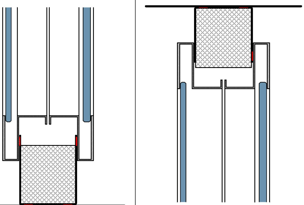
**Glazed partition, laminated glass 33.2 + laminated glass 44.2, glasses framed in profile, height horizontal profile 50mm**
