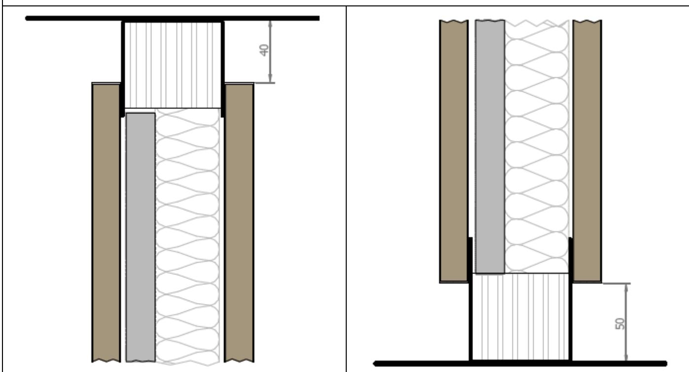
**Opaque partition, 18mm thick particle board panels, wooden top and bottom chock, one-sided acoustic membrane**
