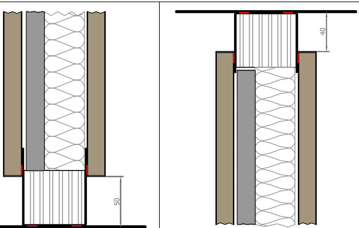
**Opaque partition, 18mm thick particle board panels, Antivlam, wooden top and bottom chock, gypsum board 18mm**
