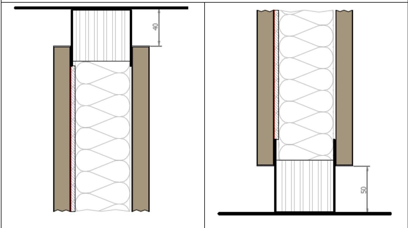
**Opaque partition, 18mm thick particle board panels, wooden top and bottom chock, two-sided acoustic membrane**
