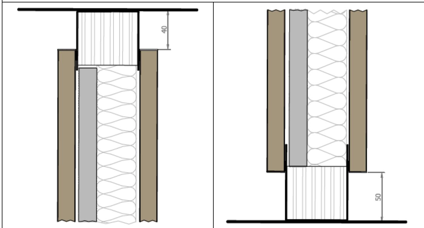
**Opaque partition EI 30, 18mm thick particle board panels Antivlam, gypsum board 18mm, wooden top and bottom chock**
