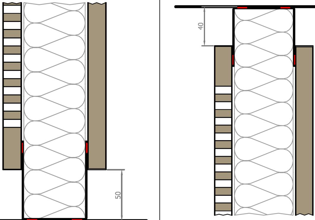
**Opaque partition, perforated MDF 18mm / cavity / perforated MDF 18mm**
