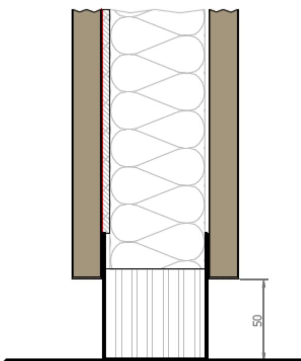
**Opaque partition, 18mm thick particle board panels, Antivlam, wooden top and bottom chock, one-sided acoustic membrane**
