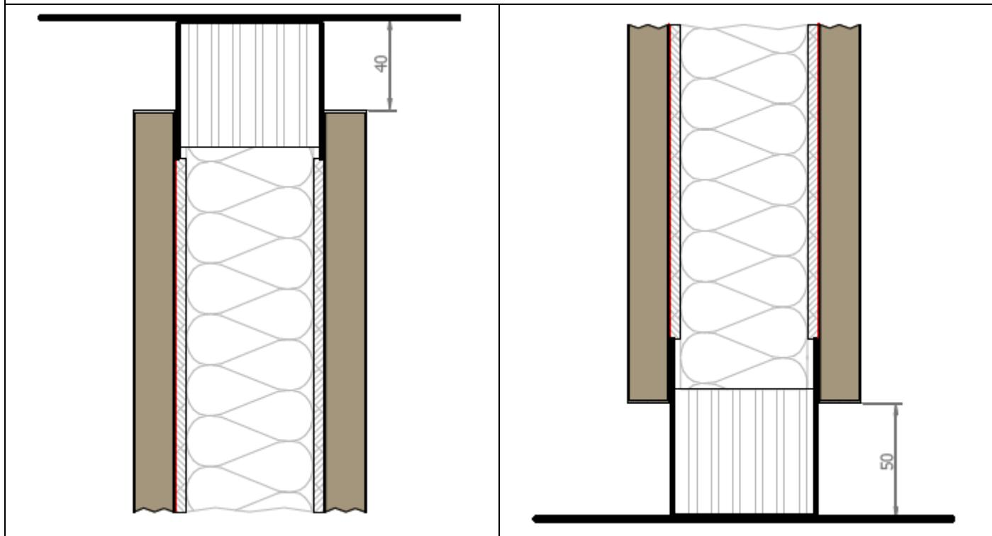
**Opaque partition, 18mm thick particle board panels, antivlam, wooden top and bottom chock, two-sided acoustic membrane**
