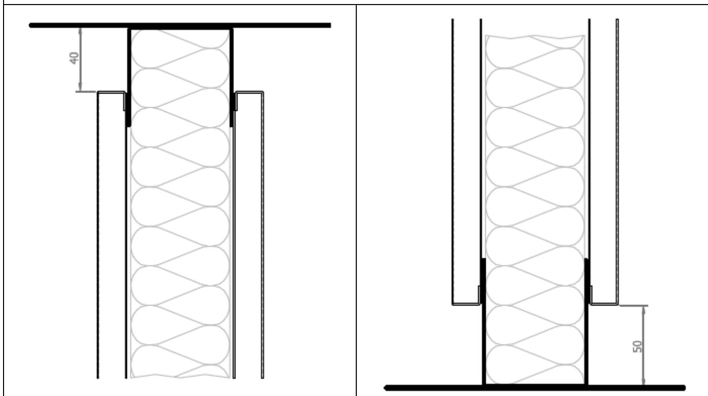
**Opaque partition, perforated cassette steel 1mm / cavity + Gypsum board 12,5mm / perforated cassette steel 1mm**
